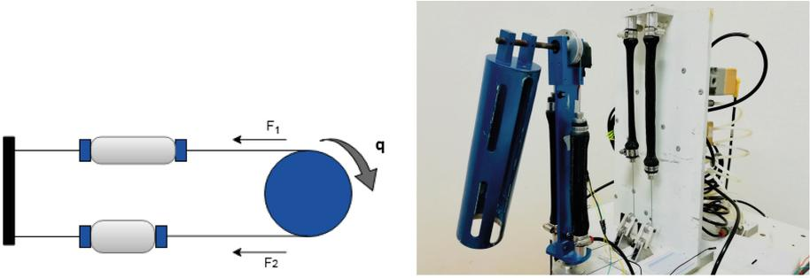
**Fig. 1.** One DoF McKibben artificial muscle scheme (left) and the experimental setup that will be used for experiments (right)
