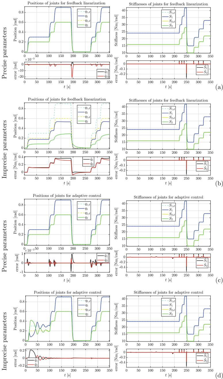
**Fig. 2.** Positions and stiffnesses of joints for feedback linearization approach with precise (a) and 1% imprecise (b) dynamic parameters, and adaptive approach with precise (c) and 1% imprecise (d) parameters
